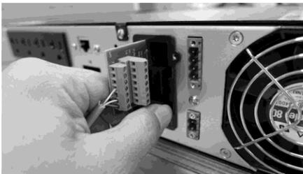
4. Connect the cable, then screw the cover as following pictures.
